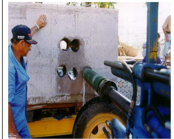
**Drilling cores from the RCC block**
