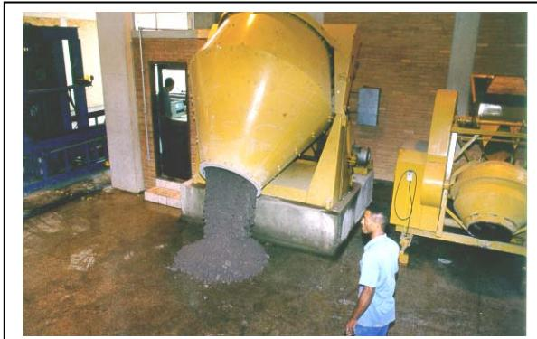
**RCC Production at Laboratory with large size mixer 1,5m<sup>3</sup> capacity**
