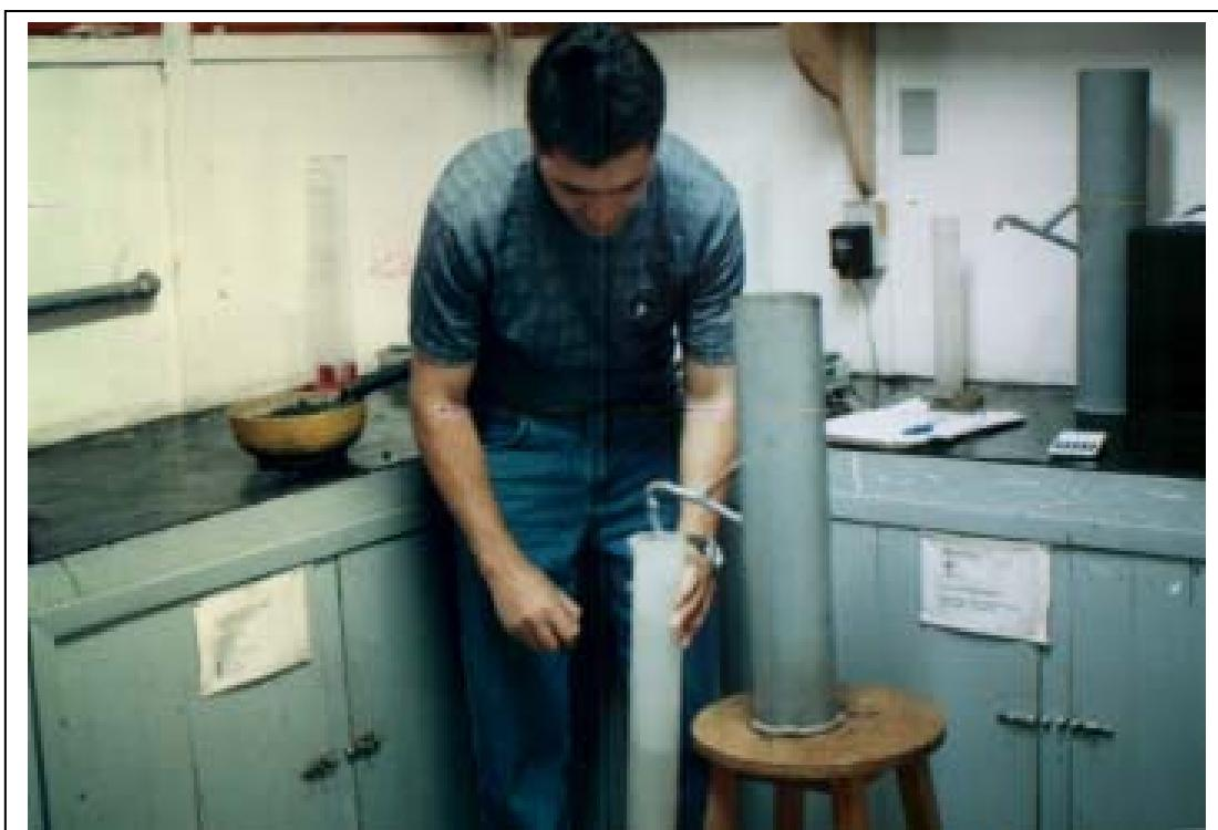
This method has been conceived based on a physical principle, the density of materials compounding concrete. Water being a material with lower density, the more water in a RCC mix, the lower the density.
