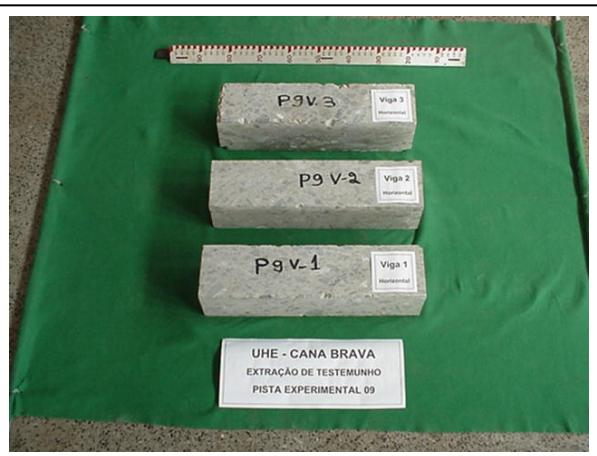
**Drilled and sawed cores from the RCC block for tests**
