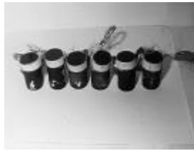
Figure 9 – Cylindrical specimens used in the compression tests
