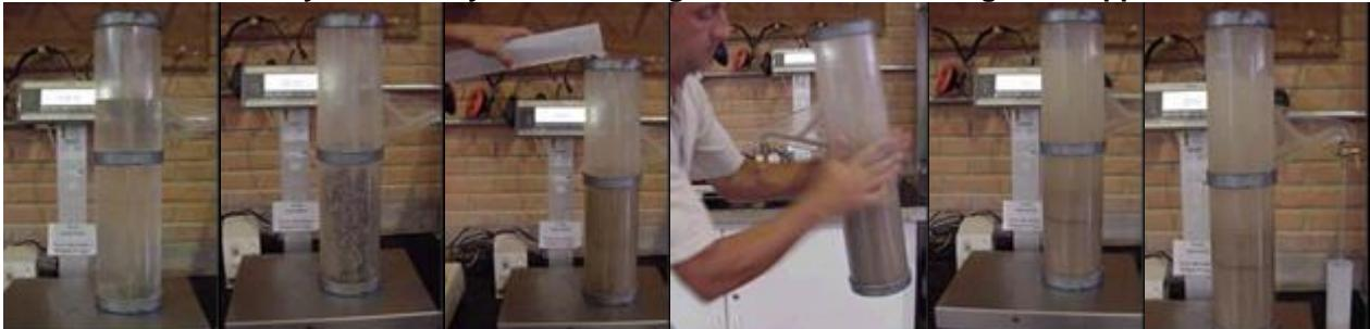
Determination of the Unit Weight and Water Content using DMA (*"Dispositivo Medidor de Agua"*- Apparatus for Water Content Measurement) apparatus, developed by Pacelli around 2003.
