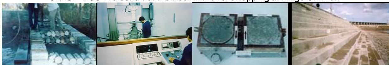
CESP- RCC trench as test fill and laboratory tests (shear) and the RCC use for Porto Primavera Dam slope Protection
