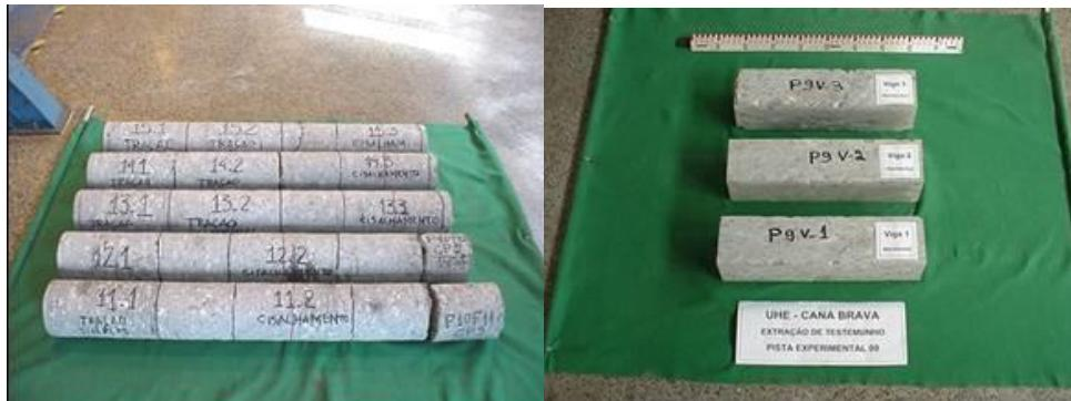
Drilled and sawed cores from the RCC block for tests
