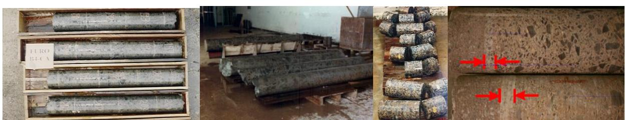
Drilled cores for test and inspection of the behavior of the construction joint and bedding mortar use
