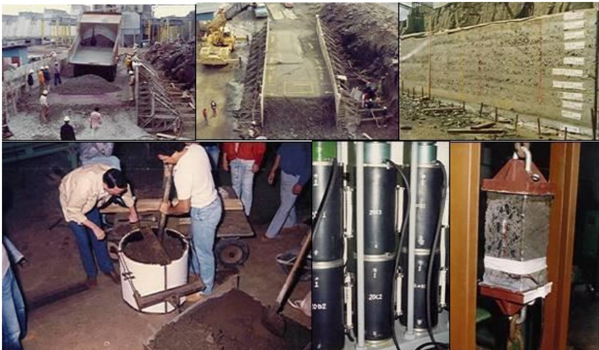
**ITAIPU- Test Fill and Laboratory tests (Adiabatic Temperature Rise; Creep and Strain Capacity) for Urugua-I (Argentina ) and Capanda (Angola) RCC Dams**
