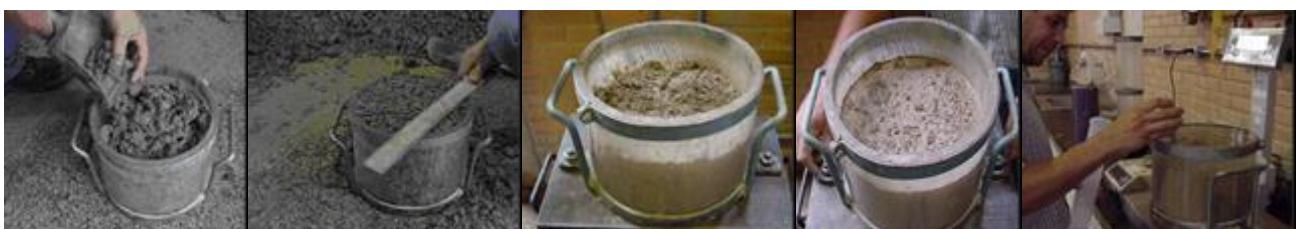
Consistency/Workability and Unit Weight determination using VeBe apparatus
