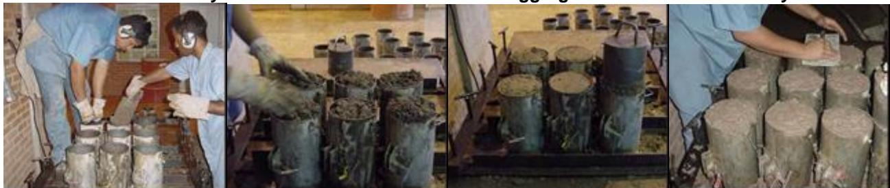
Casting cylindrical specimens with RCC
