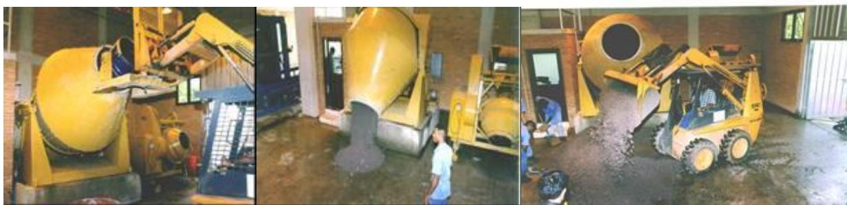
RCC Production at Laboratory with large size mixer 1,5m<sup>3</sup> capacity
