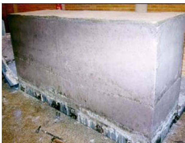
RCC test fill specimen demolded
