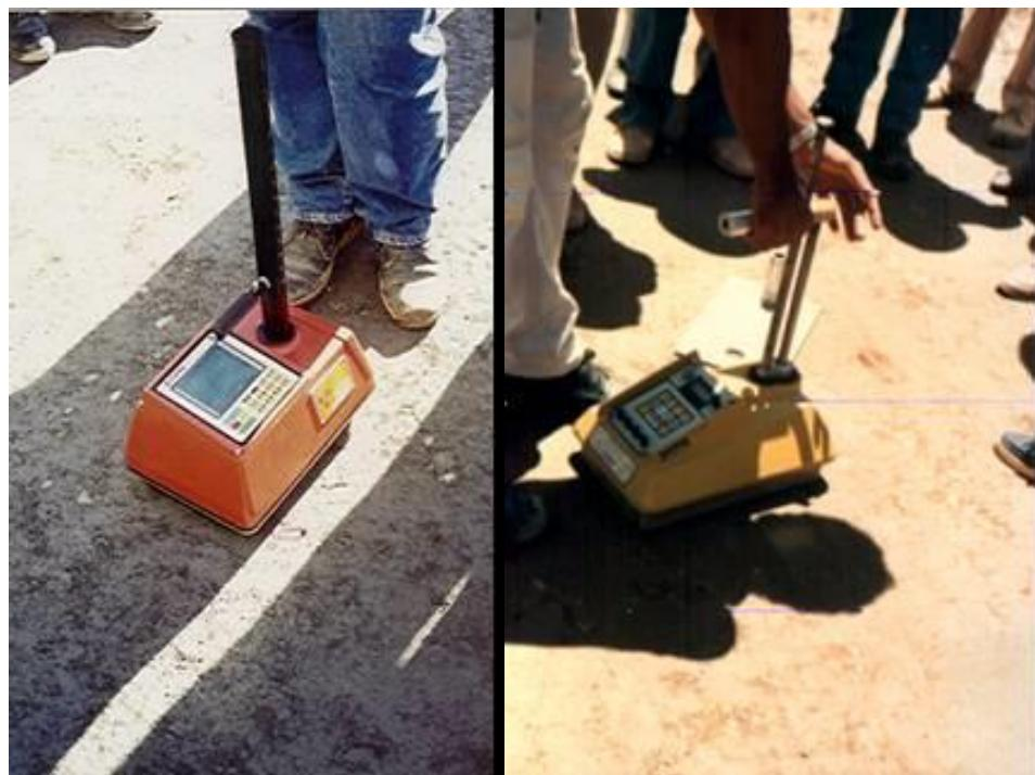
Determination of density, moisture and Unitary Water with Nuclear Densometer
